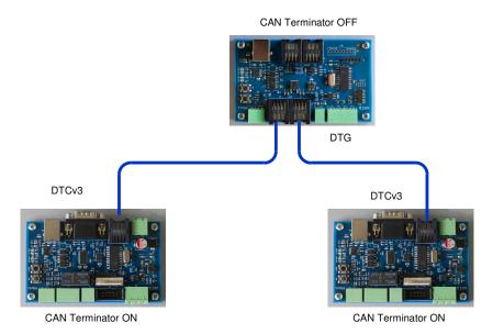
To connect two DTC modules to a DTG, repeat the game from section 3.2. The difference here is: Since the DTG is connected with both RJ45-CAN connectors, it is NOT on the end of the CAN bus and so the CAN terminator is OFF.
