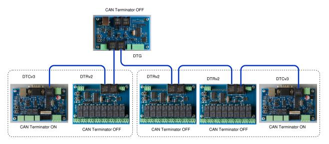
The diagram above shows a grouping, which DTR modules belong to which DTC. **NOTE:** This grouping is determined solely by configuration and is not influenced by the order in which you connect the modules.
