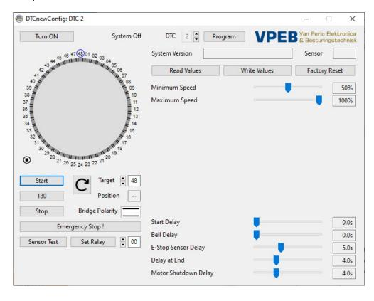
**Note:** If you change the address of a DTC, it changes only after you reset (or turn off and on) the relevant DTC module. The reason is that otherwise the address could change while you are configuring and that would lead to strange behaviour. Also, DTCnewConfig continues
