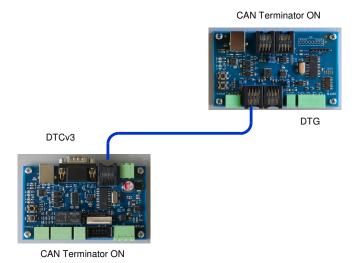
**NOTE** that power for the DTG module is supplied by the DTCv3 module and that the DTCv3 is set to supply power to the CAN bus. If you connect a USB cable from your PC to the DTG module, the blue LED on the USB interface will light up. However, the DTG only works when the red LED on the DTG module also lights up!
